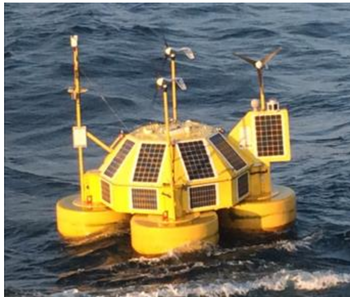
Figure 2: EOLOS Metocean Buoy as deployed.
