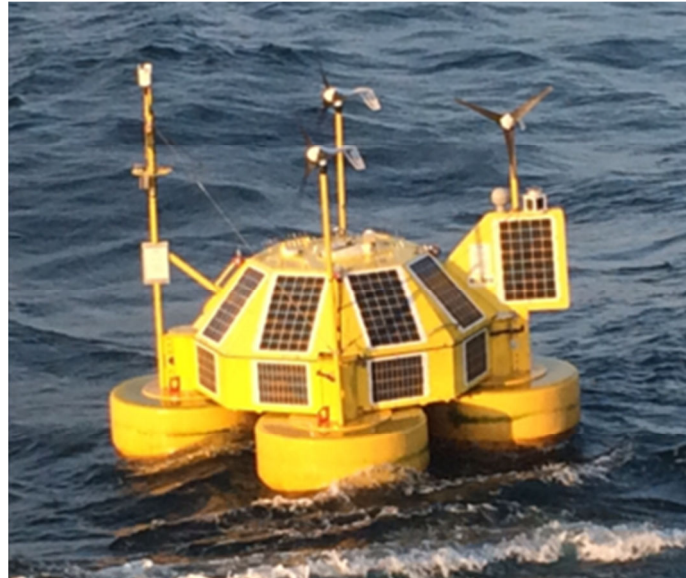
Figure 2: EOLOS Metocean Buoy as deployed.
