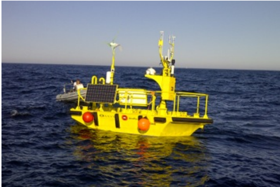
Figure 1 FLiDAR WindSentinel meteocean buoy as deployed.
