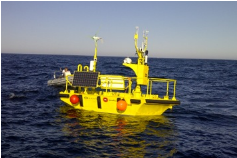
Figure 3 - FLiDAR WindSentinel metocean buoy as deployed.
